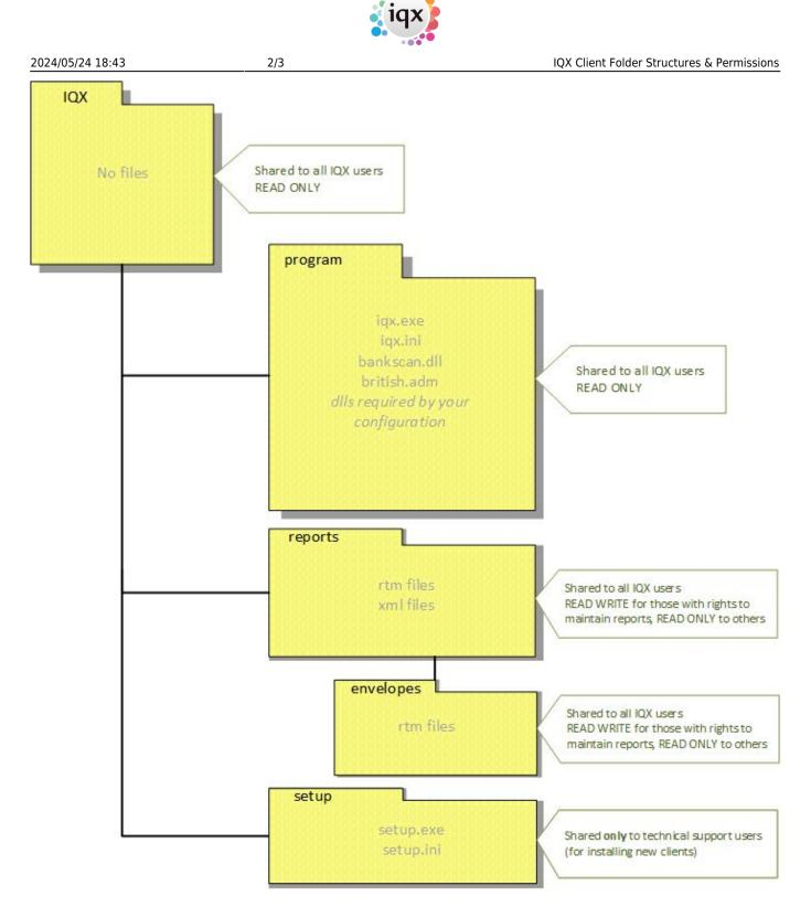
with the base folder shared as \\ApplicationServer\IQX The location chosen for the shared folder SHOULD NOT normally be on the database server but on a file or application server accessible by normal users. There is then no need then for users to have a login to the database server machine.
